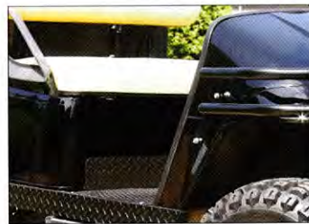
605394 KICK PLATE BLACK DIAMOND PLATE Fits all E-Z-GO vehicles including, 1982-current Marathon, TXT, RXV, Medalist, ST 350, Clays Car, 2+2, 6-Seater Carriers, and 4 Caddy Vehicles
