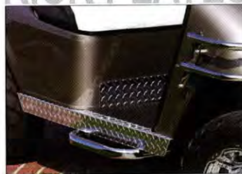
605393 KICK PLATE BRIGHT DIAMOND PLATE Fits 1994-current TXT, Medalist, RXV, Clays Car, 2+2 and 6-Seater Carriers, and 4 Caddy Vehicles
